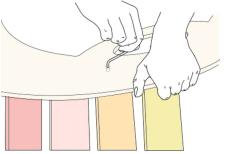
12. After all the slats are in the sockets tighten the screws all the way.
