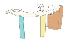
6. Hold with your hand and fix the middle slat in place with the screw.
