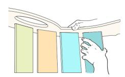
8. Place the rest of the slats in the sockets and fix them with screws.
