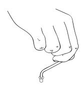
NB! Push the assembly key to the bottom of the screw head.
