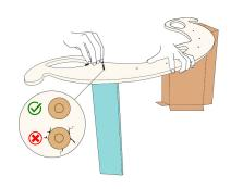
5. Lay the box vertically under the side detail. Hold in place with your hand and fix the first slat into the **socket** with the screw. **Tighten the screw all the way**.
